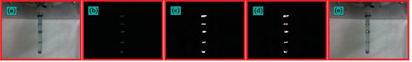
Fig. 7. Manipulator recognition via feature detection. The manipulator is labeled with three blue markers, while the proximal and distal end-effector (disk) are embedded inside the PDMS body. The image resolution is 640 \times 480 pixel. (a) RGB image; (b) gray scale image with blue elements are subtracted; (c) binarized image; (d) centroid assignment based on contour recognition; (e) labeled RGB image.
